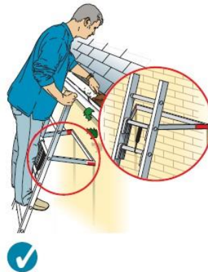
Figure 9 Stand-off device and working maximum height on a ladder
