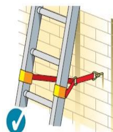
Figure 6 Tying near the base
