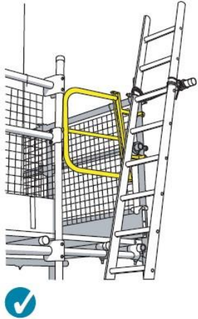
Figure 8 Access ladders should be tied and extend at least 1 m above the landing point to provide a secure handhold
