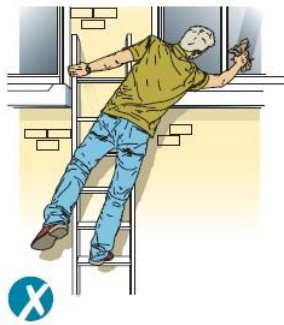
Figure 1a Incorrect - overreaching and not maintaining three points of contact
